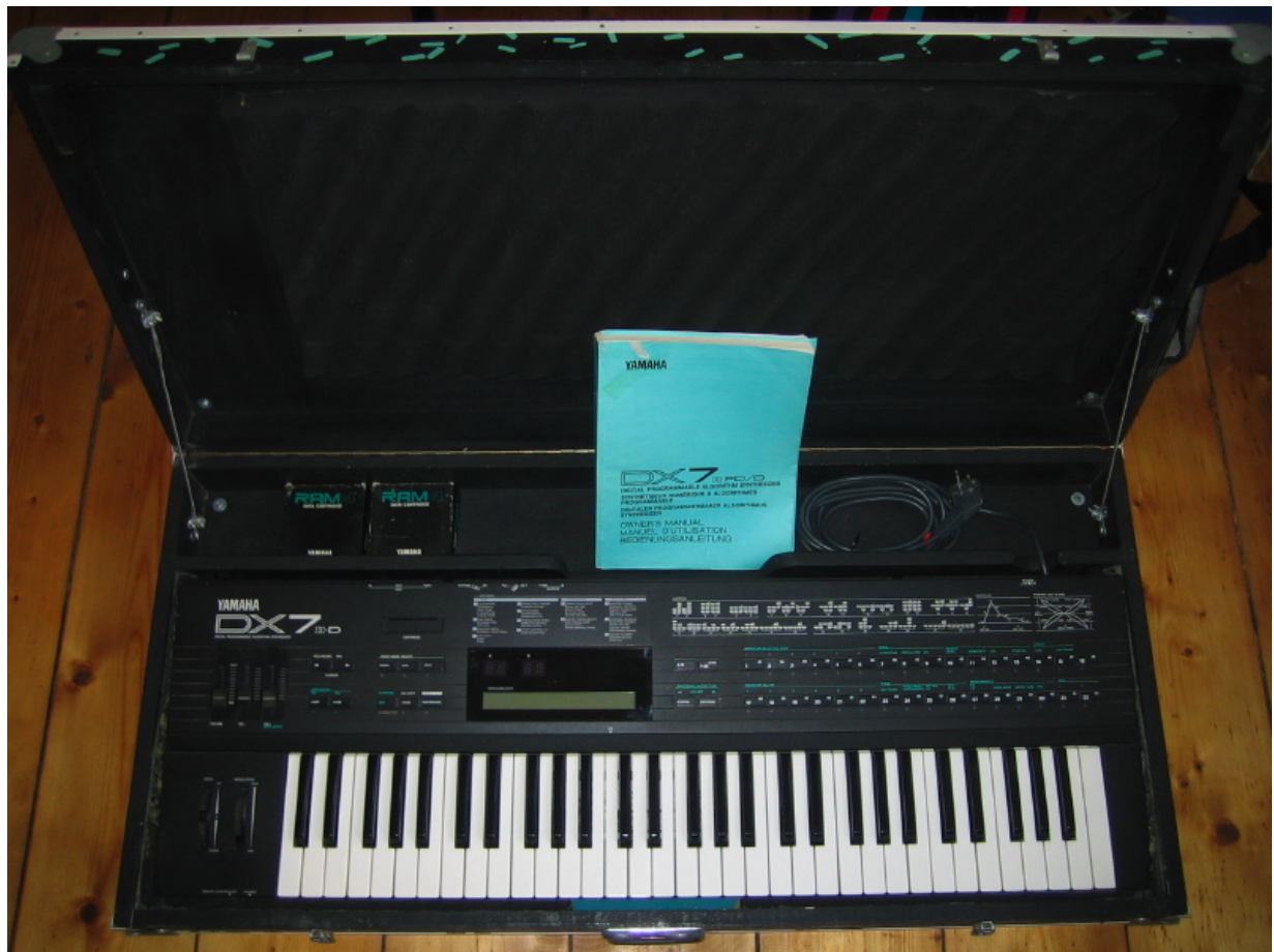
Yamaha DX7 synthesizer, the first commercially successful instrument to offer FM synthesis, digital synthesis, and MIDI compatibility. The instrument pictured here is packaged in a road case. Photographer:
